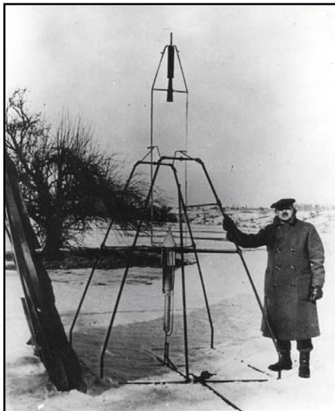
**Fig. 1. 9. Goddard and a liquid oxygen-gasoline rocket in the frame from which it was fired on March 16, 1926, at Auburn, Massachusetts. (Courtesy NASA; <http://grin.hq.nasa.gov/UTILS/search.cgi> )**
