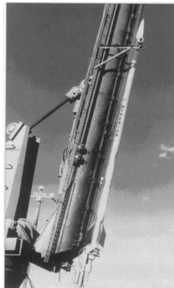
**Fig. 4 Successful hybrid rocket flight using Hyperion launch vehicle. A flight in April 1997 reached an altitude of 34 km. The hybrid rocket used nitrous oxide and HTPB as propellants (adopted from Ref. 9).**
