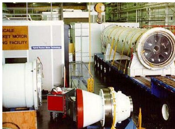
**Fig. 8 Hybrid motor assembly at NASA- Marshall — note the wagon wheel grain configuration for the fuel grain (adopted from [www.nasa.gov](http://www.nasa.gov)).**
