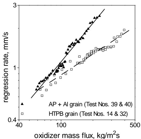
**Fig. 7 Regression rates of HTPB grains with initial port diameter = 20 mm and AP + Al grains with initial port diameter = 12 mm.**<sup>18</sup>
