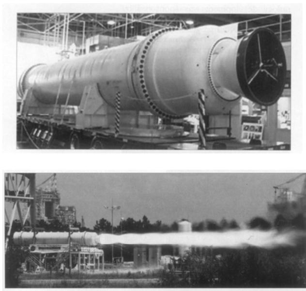
**Fig. 5** The 1.1 MN thrust turbo-pump fed LOX/HTPB hybrid motor (the third in the series) is being tested at NASA-Stennis on September 9, 1999. The motor is 13.7-m long, 1.78-m diameter, and weighs about 56800 kg. The test duration was 38 s (adopted from Refs. 10 and 11).
