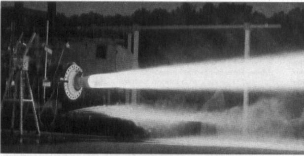
**Fig. 3 The submerged flex-bearing thrust vector control ( $\pm 4^\circ$ ) on a 610-mm (24") diameter, 53.5 kN (12000 lbf), 20 s, LOX/HTPB/Escorez hybrid motor at NASA-Marshall (Adopted from Ref. 7).**
