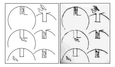
Fig. 1. 7. A duplicate copy in the left for better image-clarity and the copy of the original drawing of Tsiolkovski showing the cosmonaut with a space suit using an airlock to exit a space vehicle in weightlessness(Courtesy: The Memorial House Museum of Konstantin E.Tsiolkovsky; <u>http://www.informatics.org/museum/tsiol.html</u>).
